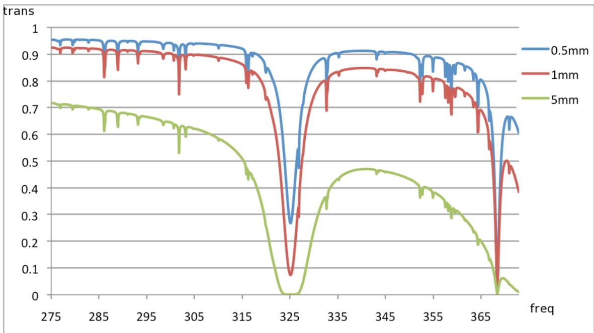
Figure 13. Band 7 atmospheric zenith transmission for  $pwv=0.5, 1.0$  and  $5.0mm$ . Frequency is in GHz.
