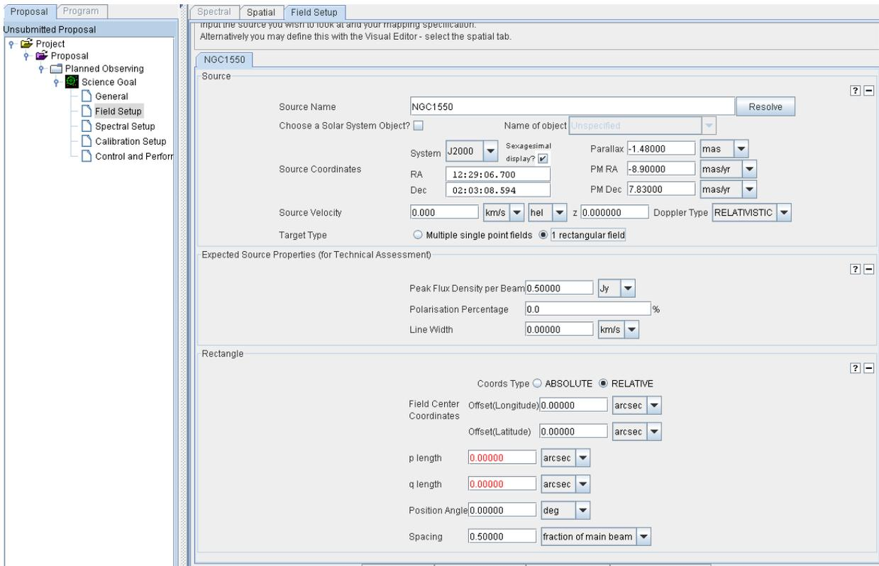
*Figure 53. Snapshot of the OT Field Setup tab showing an example of the fields that need to be used to define a rectangular mosaic field.*
