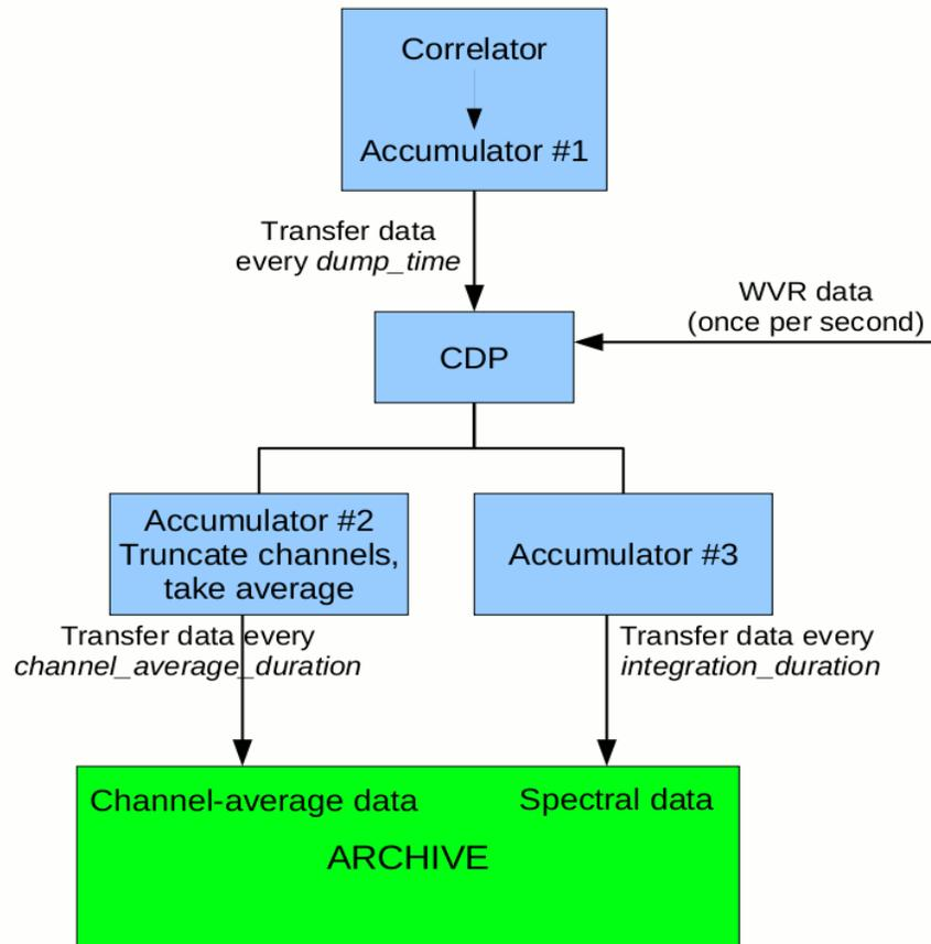
Figure 25. Data processing and accumulation steps in the correlator and archive. The timing intervals shown are described in the text.
