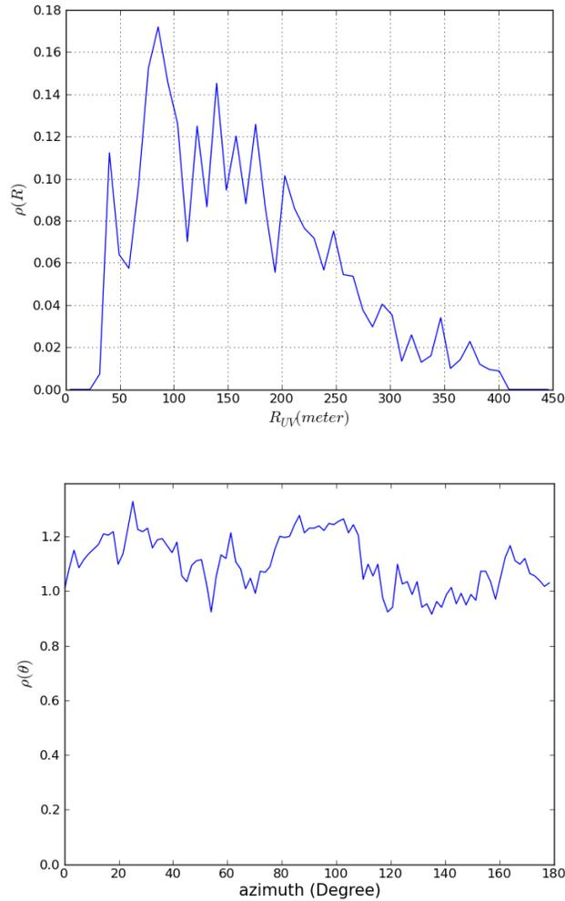
*Figure 35. Radial (top) and azimuth (bottom) density distribution of the data points in the uv-plane, normalized to the total number of visibilities during the observation, for a source with a declination of -30 degree and 6 hours of observation (+/- 3 hours in HA).*
