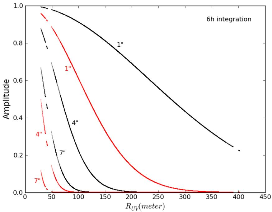
Figure 37. Sampling of Gaussian sources of different sizes (FWHM: 1", 4" and 7") with the Extended Configuration. Black lines are for Band 3 observations at 100 GHz and red lines are for Band 6
