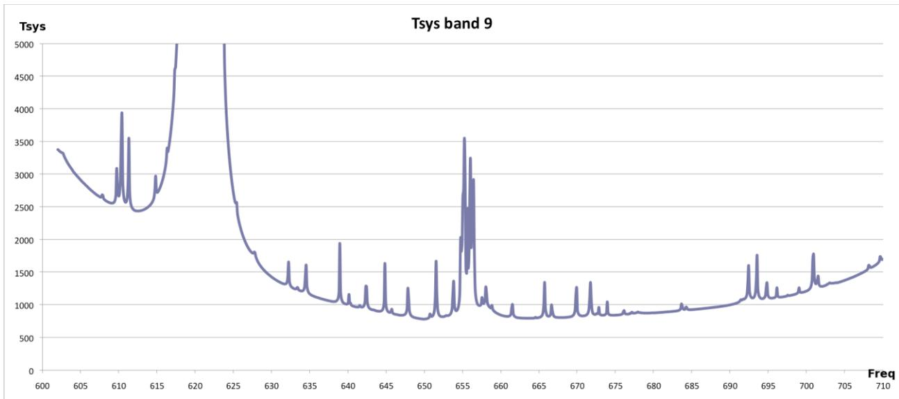
Figure 17. Typical  $T_{\text{sys}}^5$  at zenith for Band 9 with  $p_{\text{wv}}=0.5\text{mm}$ .
