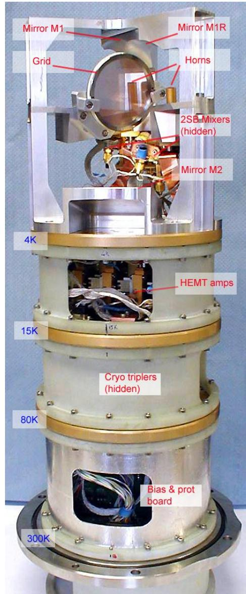
Figure 12. Band 7 frontend receiver block diagram, and (right) annotated image of the Band 7 cartridge. Note the polarization-splitting grid and LO injection in the cold optics above the mixers. The Band 7 cartridges were built at IRAM in France.
