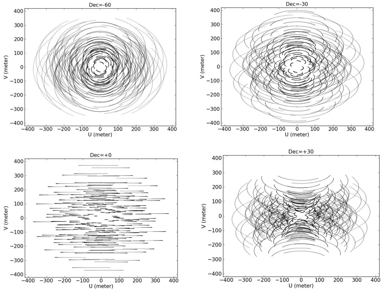
*Figure 36. uv-plane coverage for a source observed during 6 hours ( $\pm$  3 hours in HA) with a Dec= -60, -30, 0 and +30 degrees.*
