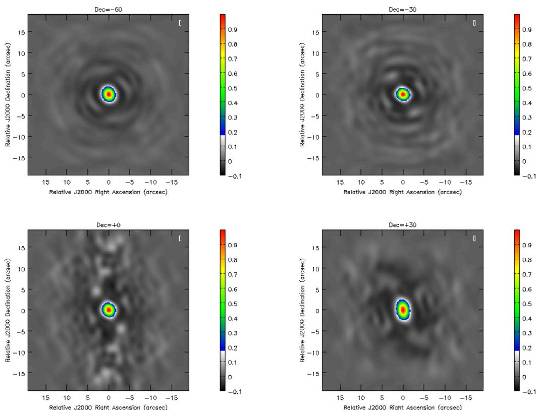
*Figure 33. Beam shape of the Cycle 0 Compact Configuration for a source at Dec= -60, -30, 0, +30 degrees observed at a frequency of 230 GHz for a duration of 6 hours (+/- 3 hours in HA).*
