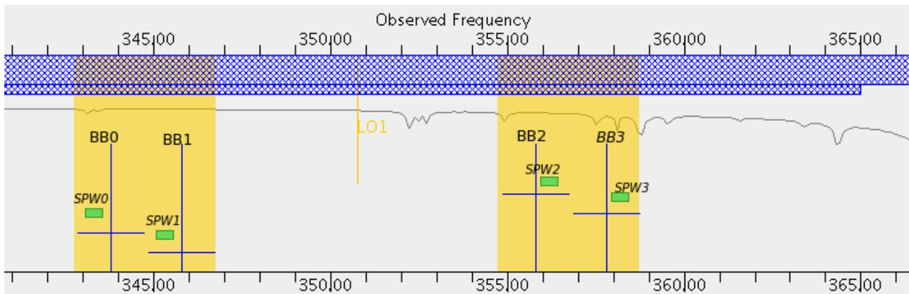
Figure 26. Illustration of a frequency setup, based on the OT spectral display. Yellow areas are the IF ranges, blue crosses are the 1.875 GHz-wide basebands (BB0-4), and green rectangles represent four narrowband spectral windows (SPW0-4). The frequency of LO1 is shown by the central vertical line. The blue hashed area shows the possible tuning range of the frontend, and the curved line gives an indication of the atmospheric transmission.
