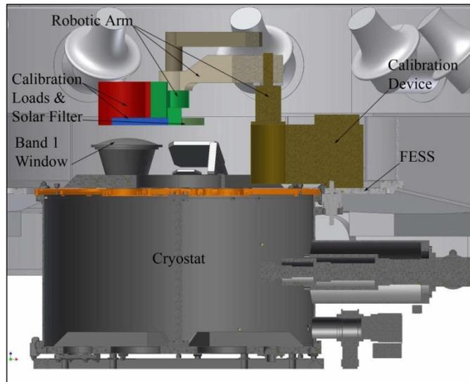
Figure 21. Lateral view of the ACD on top of the ALMA front-ends.
