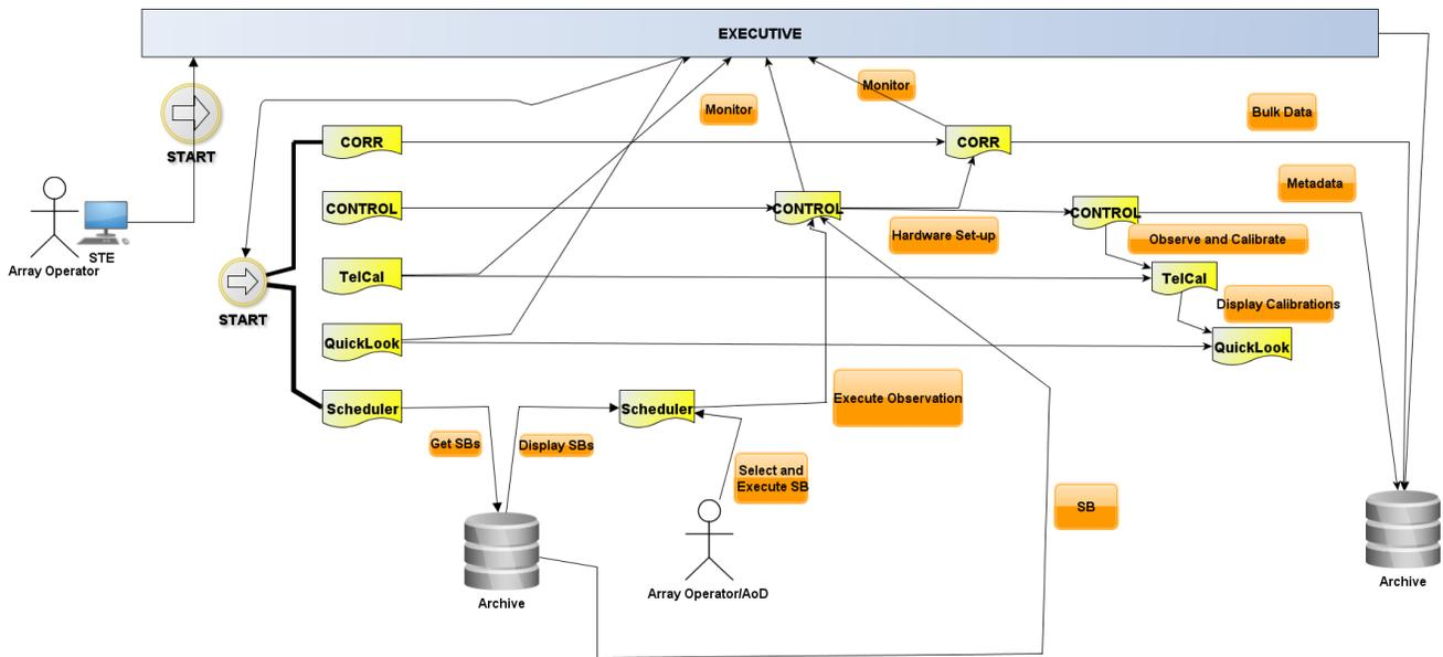
*Figure 57. Main actors and roles during observations with ALMA. The horizontal direction represents time evolution.*
