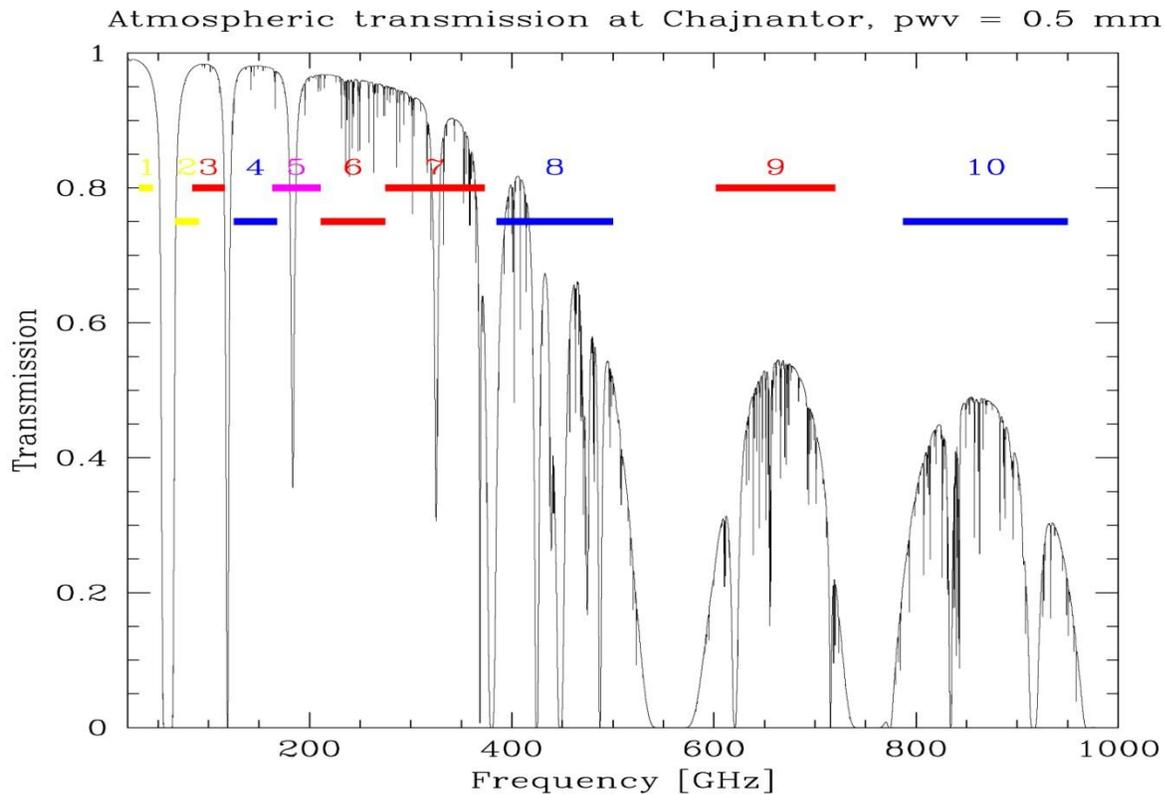
*Figure 1. ALMA Bands for Cycle 0 are shown in red superimposed on an atmospheric transparency plot at the AOS for 0.5 mm of PWV.*
