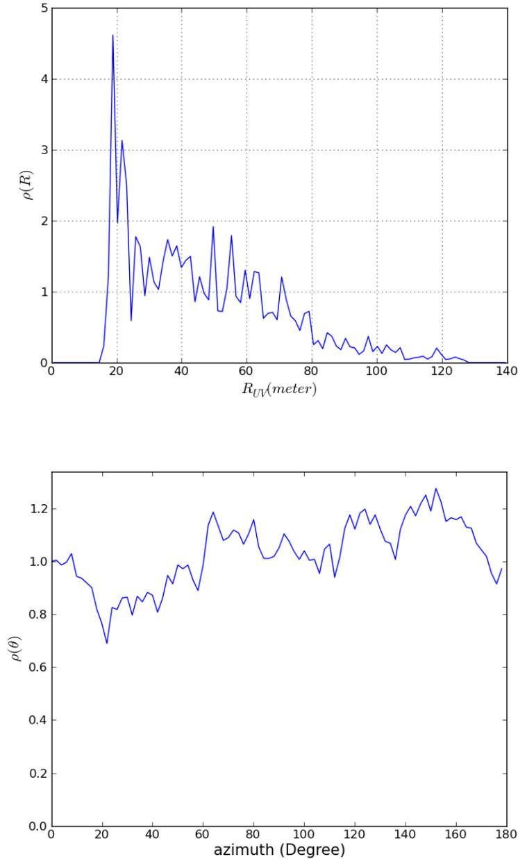
Figure 30. Radial (top) and azimuth (bottom) density distribution of the data points in the uv-plane, normalized to the total number of visibilities during the observation, for a source with a declination of -30 degrees and 6 hours of observation ( $\pm 3$  hours in HA).
