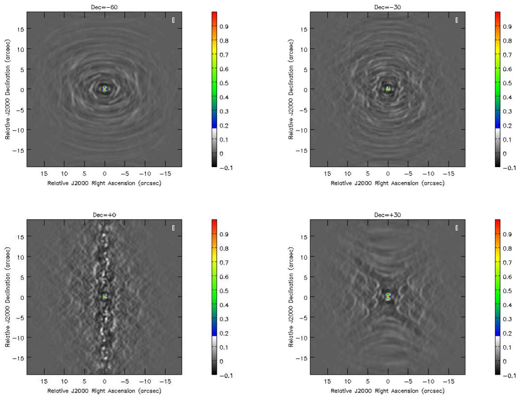
Figure 38. Beam shape in the Extended Configuration for a source observed during 6 hours ( $\pm 3$  hours in HA) with a Dec = -60, -30, 0, +30 degrees ( $f = 230$  GHz).
