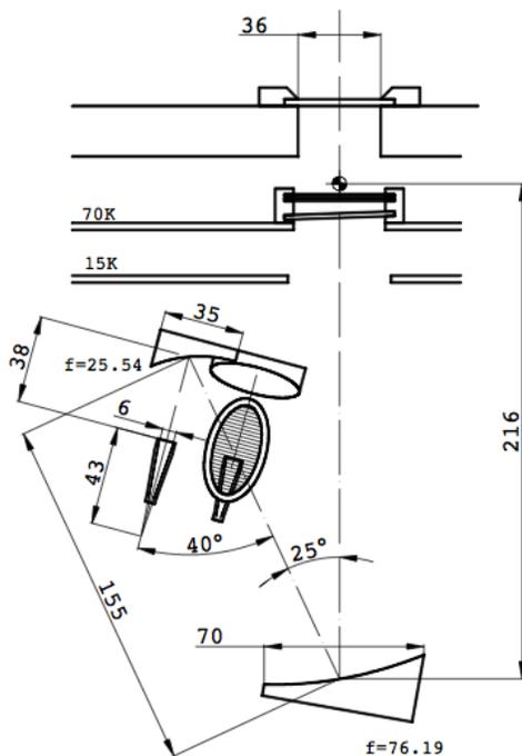
Figure 11. Band 7 cold optics arrangement, showing the off-axis ellipsoidal mirrors and the polarization splitter wire grid.
