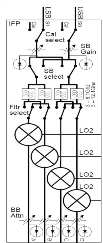
Figure 72. Block diagram of IF Processor.
