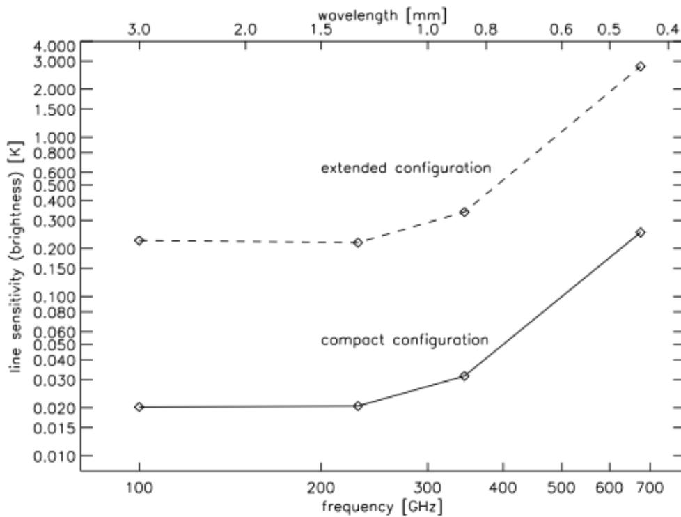
Figure 43. Line sensitivity, defined as 3 times the noise RMS, for a 3 km/s line width that can be achieved in a 4 hour observation.
