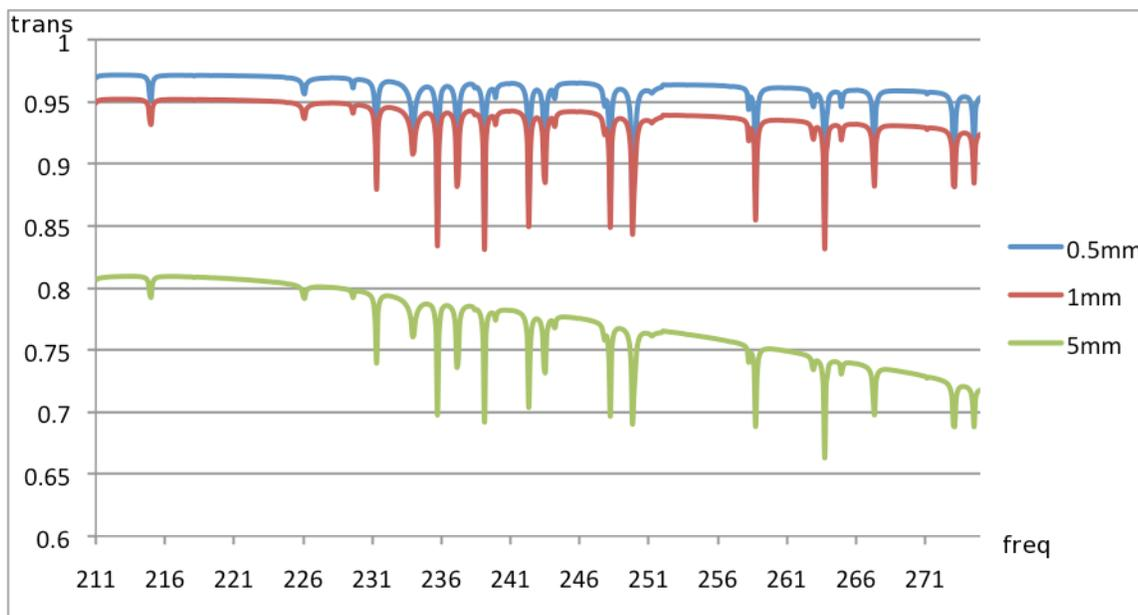
Figure 9. Band 6 zenith transmission for pwv=0.5, 1 and 5mm. Frequency is in GHz.
