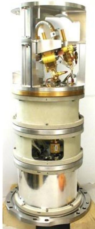
Figure 8. Band 6 receiver block diagram, and (right) image of cartridge. Note the OMT used to split the polarizations feeding the two 2SB mixers. The LO around 80 GHz requires an extra x3 multiplier inside the cryostat. The Band 6 cartridges are built at NRAO, Charlottesville. Note that the IF output range is actually 5-10 GHz. The range shown is the one recommended for continuum observations (see text)
