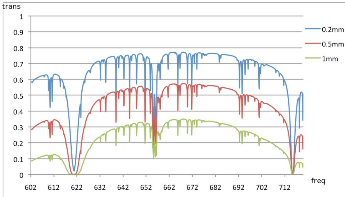
Figure 16. Band 9 zenith transmission for pwv = 0.2, 0.5 and 1mm. Frequency is in GHz.
