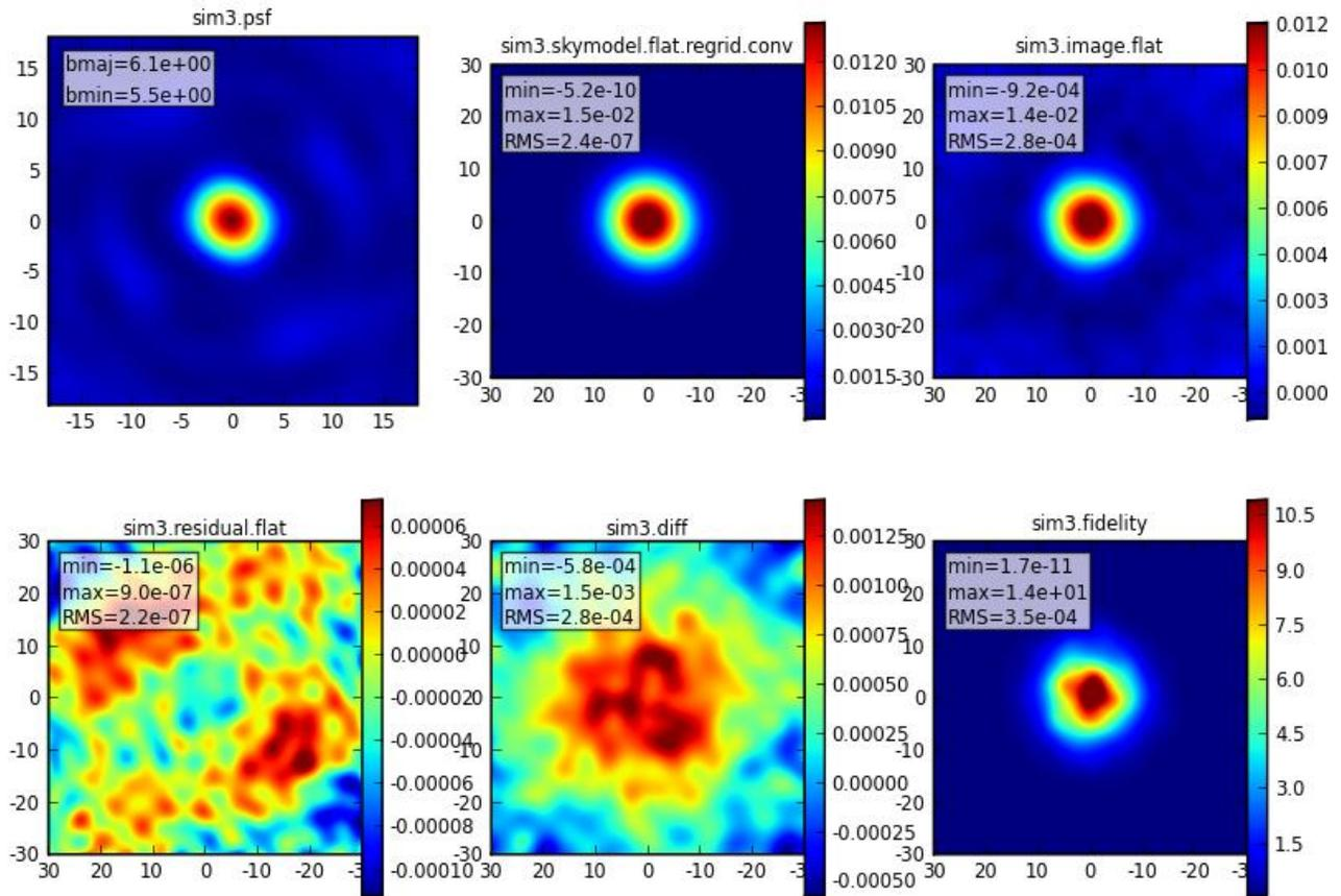
Figure 45. Simulated observation of a 10 arcsec (FWHM) Gaussian with a dynamic range of 100 (peak flux density over rms noise) in the compact configuration at 90 GHz. The panels for output images can be configured, and here they are (from top left to the right and bottom left to the right): Synthesized beam, convolved input model, CLEANed output, CLEAN residuals, difference map (input-output) and image fidelity. All axes are in arcsec.
