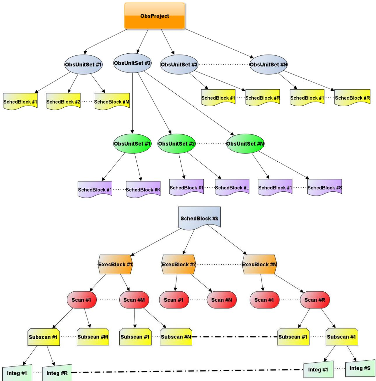
Figure 56. Block diagram of an Observing Project from the point of view of the observation preparation (top) and actual execution (bottom). Note that an ObsUnitSet can be composed of other ObsUnitSets as explained in the text. Each time an Schedblock is executed, CONTROL creates a new ExecBlock structure (see text).
