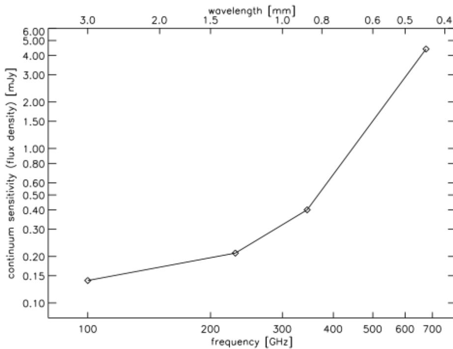
Figure 41. Flux density continuum sensitivity, defined as 5 times the noise RMS, that can be achieved in a 1- hour observation.
