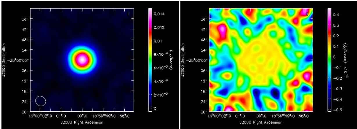
Figure 46. *Msclean* deconvolution in CASA of the simulated observation of the 10 arcsec (FWHM) Gaussian function in Figure 45 (compact configuration at 90 GHz). The deconvolved image is on the left; the *msclean* residuals are on the right.
