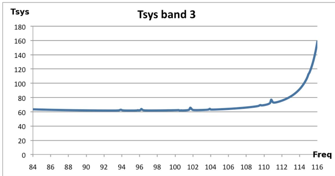
Figure 6. Typical system temperature ( $T_{sys}$ )<sup>1</sup> at zenith for Band 3 with 1mm of pwv.
