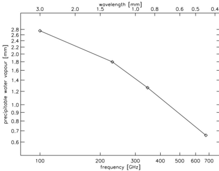
Figure 40. Precipitable water vapour (PWV) values assumed by the ALMA Sensitivity Calculator for observations in the different ALMA bands. Typically better weather conditions will be chosen for higher frequency bands.
