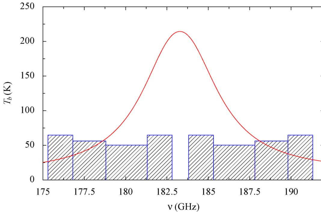
*Figure 18. WVR filters superimposed onto the 183 GHz water vapor emission line.*
