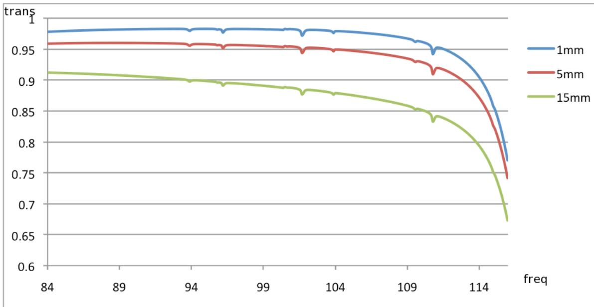
Figure 5. Band 3 transmission for 1, 5 and 15mm of pwv. Frequency is in GHz.
