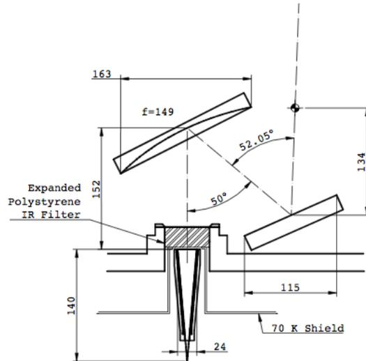
*Figure 3. Input optics for Band 3, showing the warm pickoff mirrors. The location of the antenna beam from the secondary mirror is shown by the dashed line, and the Cassegrain focus is shown by the small circle to the upper right. A new version of this Figure is being prepared by the FE group.*
