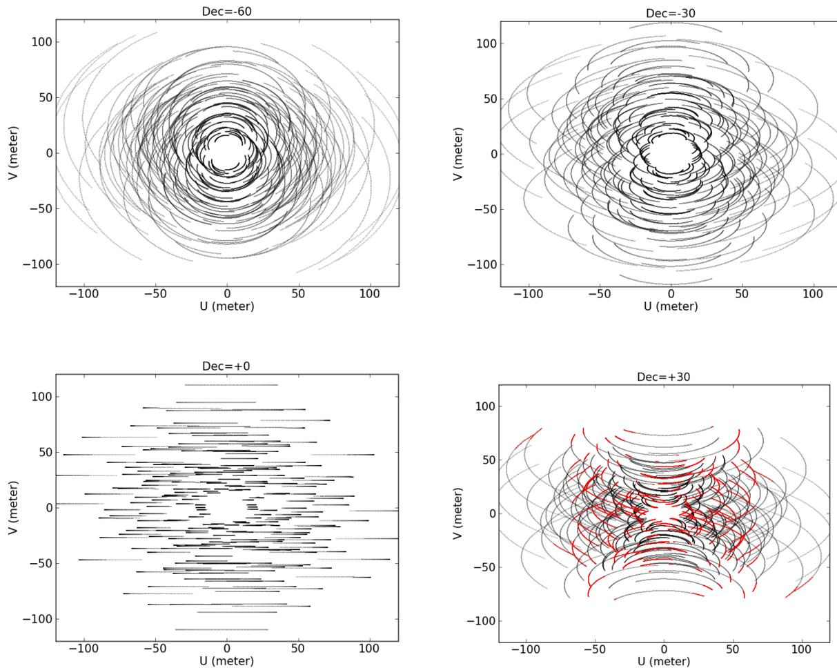
*Figure 31. uv-plane coverage for a source observed during 6 hours ( $\pm 3$  hours in HA) with a Declination of -60, -30, 0 and +30 degrees (shadowed visibilities are rendered in red).*
