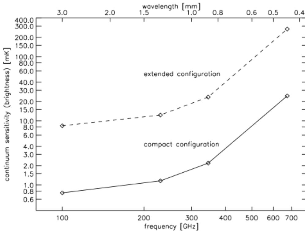
Figure 42. Brightness continuum sensitivity, defined as 5 times the noise RMS, that can be achieved in a 1 hour observation.
