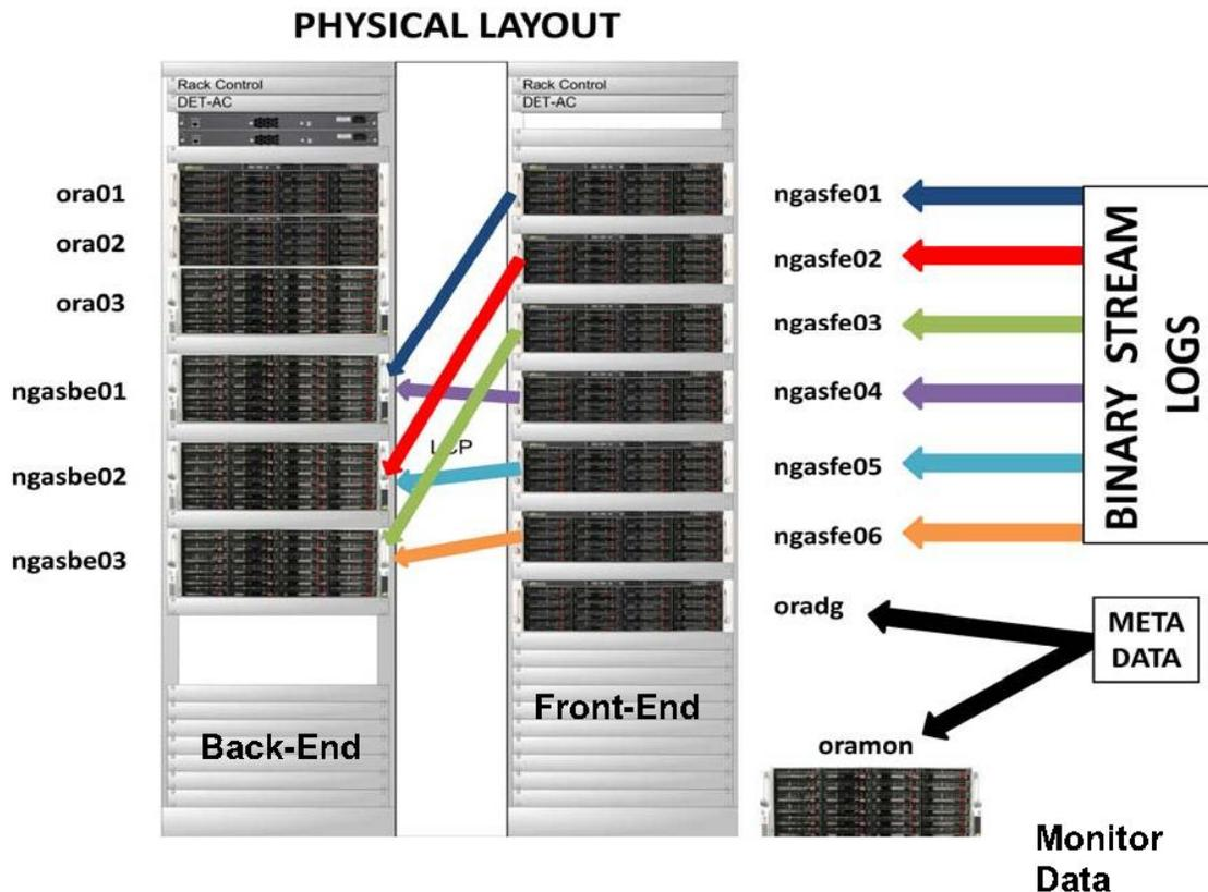
Figure 61. Archive design (front-end & Back-end) at the OSF to store metadata and raw and monitor data.
