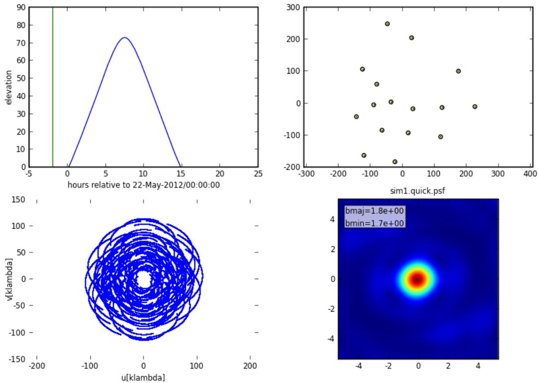
Figure 44. The output (example from simdata) gives the source elevation, the antenna positions, the uv-tracks and the synthesised beam in arcsec (here for the extended configuration). This is a 6 hour track around transit ( $\pm 3$  hours) for a source at Dec =  $-40$  deg observed in Band 3 at 89 GHz.
