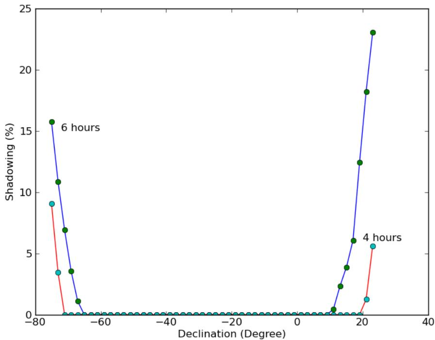
Figure 29. Shadowing fraction (the percentage of visibilities for which one antenna partially blocks another antenna's view of the target source) for a 4 and 6 hours track ( $\pm 2$  hours and  $\pm 3$  hours in HA) versus the target declination in the compact configuration.
