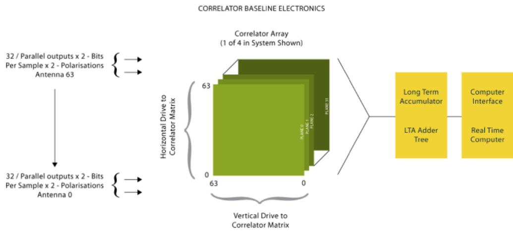
Figure 23. Diagram of the ALMA BL correlator and data transmission system.
