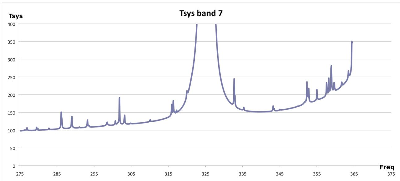
Figure 14. Typical  $T_{sys}^4$  at zenith for Band 7 with  $pwv=1mm$ .
