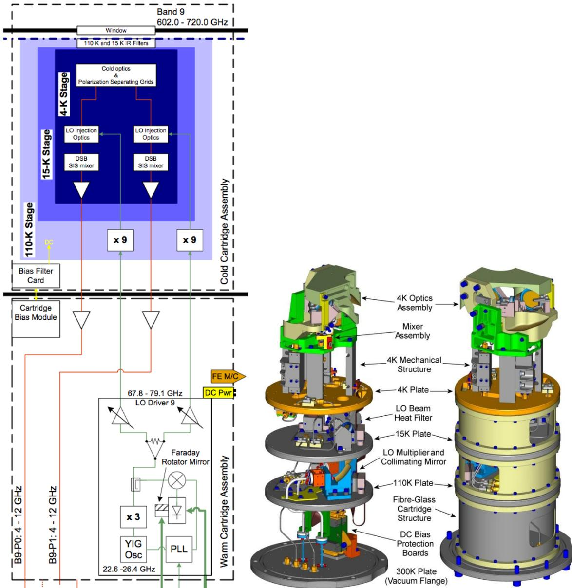
Figure 15. Block diagram of Band 9 cartridge (left) and a schematic image (right). Note that there are only two IF outputs, one from each polarization in this DSB receiver. The Band 9 receiver was built at SRON in the Netherlands.
