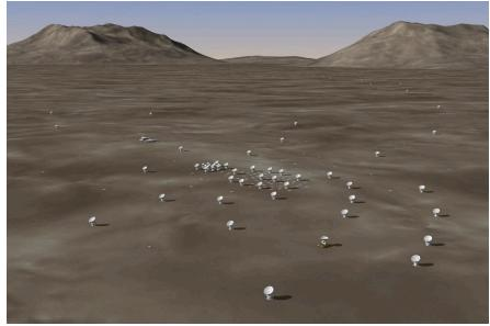
66 antennas (50 in the 12-m Array, 12 in the 7-m Array, and 4 in the TP Array). For a more detailed description of these terms, see "Interferometry Concepts for ALMA" starting on page 34.
