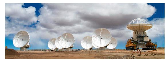
Figure 3: Another ALMA antenna takes its place at Chajnantor, carried by one of the two ALMA transporter vehicles. (Photo J. Guarda, © ALMA (ESO/ NAOJ/NRAO)
