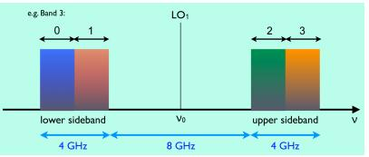
Figure 30: A graphical view of basebands and sidebands. Basebands may be tuned to overlap if the user wishes, or may be located so as to maximize the total bandwidth (as shown). Each baseband may be further subdivided into as many as 8 spectral windows. Only one spectral window per baseband will be available during Cycle 1.
