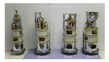
Figure 5: Four of the ALMA receiver cartridges. Eventually ALMA antennas will be equipped with at least seven receiver cartridges, covering Bands 3-10 (see Table, page 10). The Band 3 cartridges were constructed in Canada by NRC, Band 6 in the U.S. by NRAO, Band 7 in France by IRAM, and Band 9 in the Netherlands by SRON. Bands 4, 8, and 10 are being constructed in Japan by NAOJ in collaboration with U. Tokyo.
