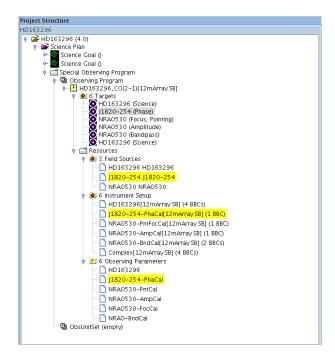
Figure 8.4: A Project Structure that contains one SB. The Target folder contains one science target and many calibration targets. In the Target folder the phase calibration target is selected and its attached forms are highlighted.
