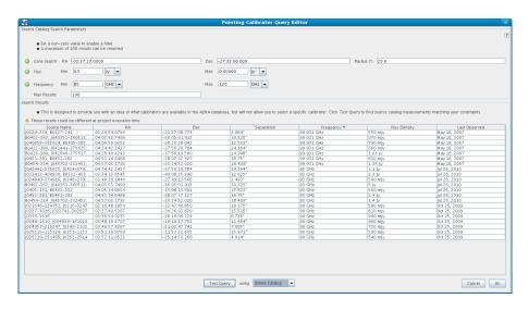
Figure 5.4: The Calibrator Selection Tool as used in the Calibration Setup of Science Goal. A search has been made for all calibrators within a 10-degree radius of a source position, that have a flux greater than 500 mJy in ALMA Band 3.
