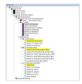
Figure 8.13: A Phase 2 observing program structure that contains one Scheduling Block. The Scheduling Block contains 5 Targets. Field Source, Instrument Setup and Observing Parameters forms have been created in the Resources folders. The figure shows the highlighted target HD163296 in the Target folder and the attached parameter sets.
