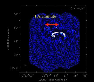
Figure 22: Estimating the LAS of CO (1-0) emission in M100. We examine individual channels of the ALMA Science Verification data and look for the largest angular extent of emission in any direction. Within this channel we see contiguous emission extending at least an arcminute. This is larger than the maximum recoverable scale sampled by the main 12-m Array at Band 3, so ACA observations will be a necessary complement to the main array data.
