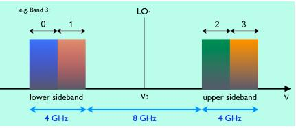
Figure 32: A graphical view of basebands and sidebands. Basebands may be tuned to overlap if the user wishes, or may be located so as to maximize the total bandwidth (as shown). Each baseband may be further subdivided into as many as 8 spectral windows. Up to four spectral windows per baseband will be available during Cycle 2.
