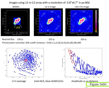
Figure 16(b) [below]: *Here we show* simulated observations of a source which has structure only on small spatial scales, such as a cluster of compact galaxies or protostars (top left). The LAS is wellwithin the range of the shorter 12-m Array baselines.
