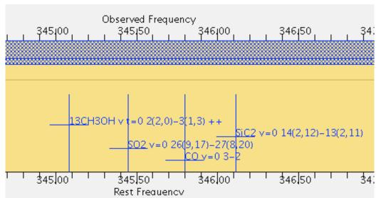
Figure 35: Four spectral windows were set up to observe these four lines simultaneously in one baseband using the OT. The windows are each 234 MHz wide (with 0.43 km/s channels), and are centered at 345.80, 345.45, 346.11 and 345.09 GHz. The spectral windows must fit within the 2 GHz wide baseband.
