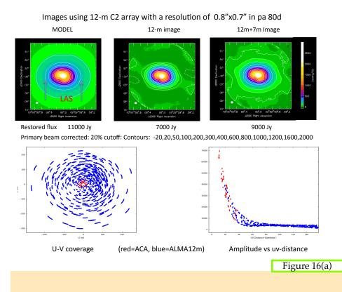
Observing sources with a range of spatial scales (such as power-law envelopes) requires careful consideration of the effects of finite baselines and the respective *uv*-coverage as shown by the following analysis of reconstructed maps of complex regions. These simulations were generated using the CASA *simalma*. The largest angular structure (LAS) of structure is shown by the arrows in the model image (top left image in Figures 16(a) and (b).
