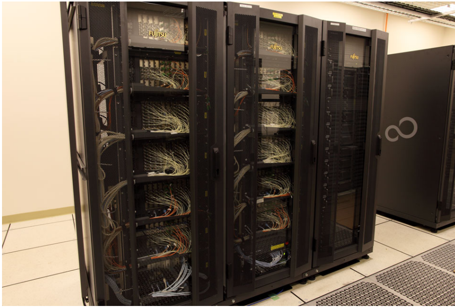
Figure 5.4: Two quadrants of the ALMA Compact Array (ACA) correlator installed in the ACA correlator room. Credit : ALMA (ESO/NAOJ/NRAO), S. Okumura
