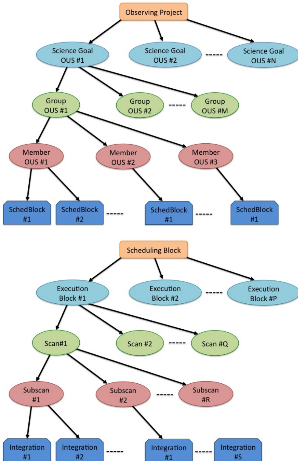
Figure 8.1: Block diagram of an Observing Project from the point of view of the observation preparation (top) and internal hierarchical structure of the Scheduling Block in actual executions (bottom). All projects have the same ObsUnitSet (OUS) levels, the Science Goal OUS level, the Group OUS level and the Member OUS level. Scheduling blocks are attached to the Member OUS. Each time a Scheduling Block is executed, Control creates a new Execution Block structure (see text).
