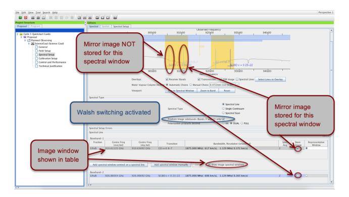
Figure 6: Spectral line observations with Walsh switching turned on, and the mirror image saved for one of the spectral windows.
