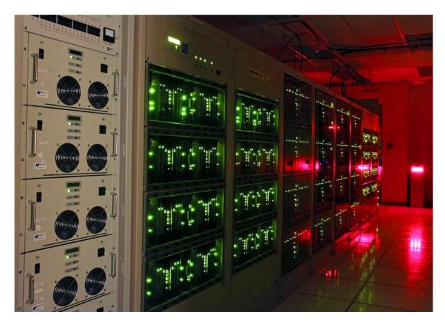
Figure 5.2: The ALMA 64-input Correlator. This view shows lights glowing on some of the racks of the correlator in the ALMA Array Operations Site Technical Building and shows one of four quadrants of the correlator. Credit: ALMA (ESO/NAOJ/NRAO), S. Argandoña
