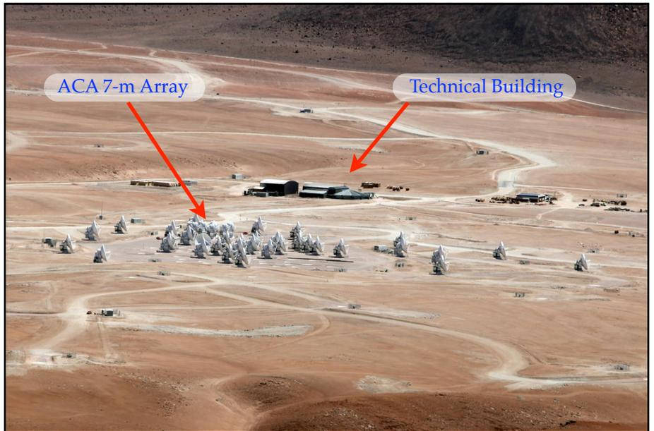
Figure 6: An aerial view of ALMA in a relatively compact configuration. The maximum distance between the 12-m Array antennas in the most compact configuration is less than 200 m, and the minimum distance a mere 15 m. Indicated also are the AOS Technical Building, and the ACA 7-m Array. (Credit: C. Padilla/ALMA (ESO/NAOJ/NRAO))
