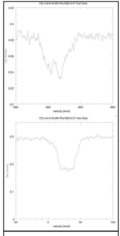
Figure 14: *Examples of molecular absorption lines detected toward PKS1830-211. These observations were made by ALMA in late 2010 when there were only a few antennas.*
