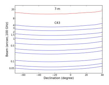
Figure 7.10: Geometrical mean of the major and minor axes of the synthesized beams as a function of source declination. These correspond to a 2-hour observation at 100 GHz and at transit. 12-m Array configurations are arranged with C43-1 at the top and C43-10 at the bottom. The 7-m Array is also shown.
