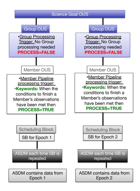
Figure 13.2: Pipeline processing of a Science Goal containing multi-epoch observations. Each epoch is processed independently by the Pipeline, with science products created for each epoch. Data from different epochs are not processed together to form a combined product (the Member OUS from each epoch are in different Group OUS). This Science Goal would result in two Pipeline processing runs, with two sets of science products archived and delivered.
