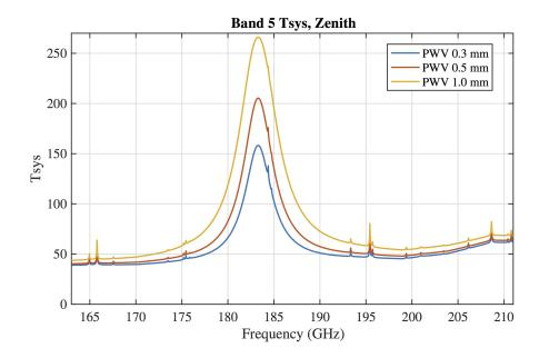
Figure 4.15: Typical system temperature  $(T_{\text{sys}})$  at zenith for Band 5 for three typical PWV values.  $(T_{\text{sys}})$  was computed using only the receiver temperature values adopted in the OT and the atmospheric contribution. No spill-over or background terms have been included. Temperature is given in Kelvin.)
