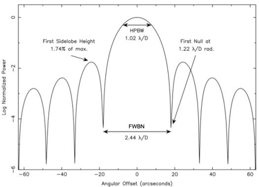
Figure 3.3: Normalized 1-D antenna power response for a 12 m antenna uniformly illuminated at 300 GHz. The power is in log units to emphasize the sidelobes. The HPBW of the primary beam is  $\sim 1.02 \lambda/D$  and the FWBN is  $\sim 2.44 \lambda/D$ . The angle of the first null, i.e., the resolution, is  $0.5 \times BWFN = \sim 1.22 \lambda/D$ . Note that the HPBW measured from actual 12 m ALMA antennas is  $\sim 1.13 \lambda/D$  because the illumination is not uniform.
