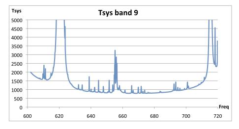
Figure 4.31: Typical  $T_{\text{sys}}$  at zenith for Band 9 with PWV = 0.472 mm.  $T_{\text{sys}}$  was computed using only the receiver temperature values adopted in the OT and the atmospheric contribution. No spill-over or background terms have been included. Temperature is given in Kelvin.
