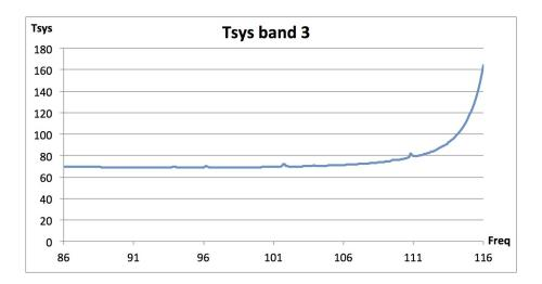
Figure 4.7: Typical system temperature  $(T_{\rm sys})$  at zenith for Band 3 with 1.262 mm of PWV.  $T_{\rm sys}$  was computed using only the receiver temperature values adopted in the OT and the atmospheric contribution. No spill-over or background terms have been included. Temperature is given in Kelvin.
