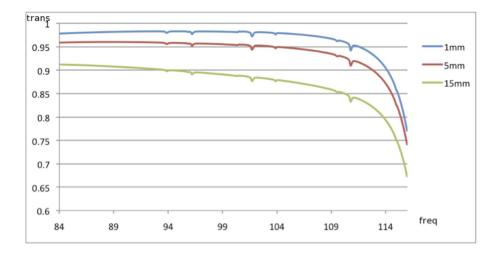
Figure 4.6: Band 3 zenith transmission for 1, 5 and 15 mm of PWV. Frequency is in GHz.
