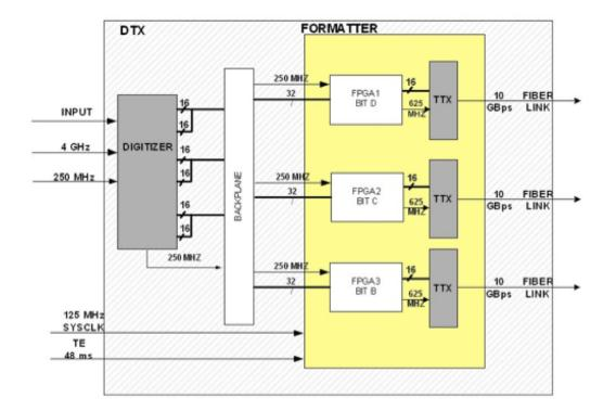
(DTX) and the receiving side at the Technical Building (DRX). Figure B.8 shows a block diagram of a single DTX module.
