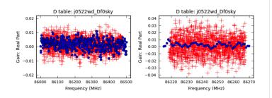
Figure 8.5: A close-up view in frequency space of the real part of D-term shown in Figure 8.4. Blue circles and red crosses are showing the *D-terms* obtained from setup #1 (FDM, 2 GHz bandwidth) and setup #2 (FDM, 500 and 62.5 MHz bandwidth respectively).
