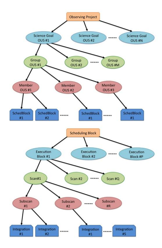
Figure 8.1: Block diagram of an Observing Project from the point of view of the observation preparation (top) and internal hierarchical structure of the SB in actual executions (bottom). All projects have the same ObsUnitSet (OUS) levels, the Science Goal OUS level, the Group OUS level and the Member OUS level. Scheduling blocks are attached to the Member OUS. Each time a Scheduling Block is executed, Control creates a new ExecBlock structure (see text).
