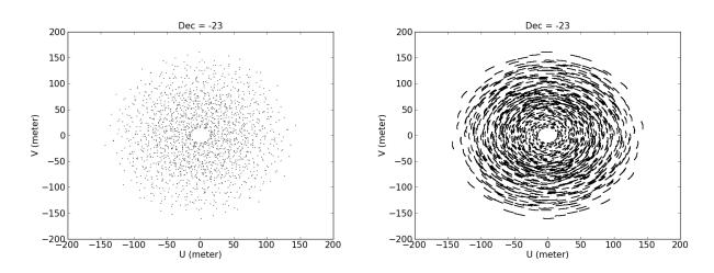
Figure 7.11: uv-plane sampling distributions of a model ALMA observation with 1-minute integration (*left*) and 1-hour integration (*right*), using the C43-1 configuration to observe a source at a declination of  $-23^{\circ}$ .
