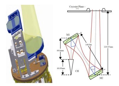
Figure 4.12: Optical layout of the Band 5. Placing the mixer assembly along the side of M 1 and streamlined layout of the IF system are the key to fulfil the requirements on  $5w_0$  optical beam clearance.
