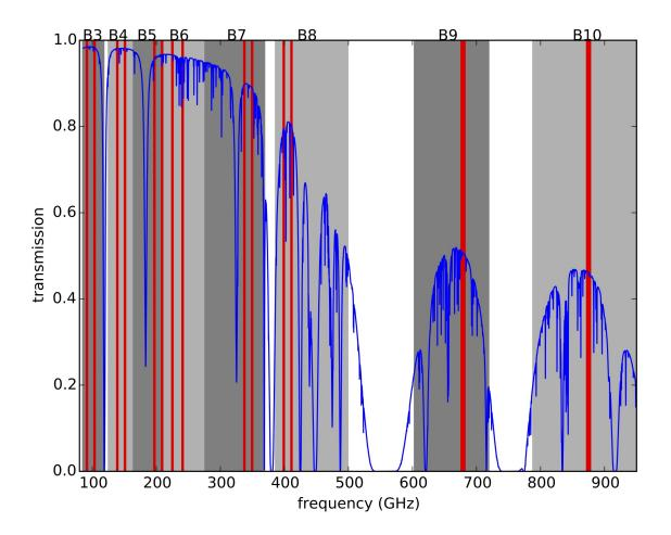
Figure 6.2: ALMA bands available in Cycle 5 (Bands 3 - 10), showing the frequency of the standard continuum settings as red shading. This gives the coverage of both USB and LSB, except for Bands 9 and 10, which have 8 GHz of bandwidth using the USB only. The available frequency coverage of each band is shown by the grey shading, and atmospheric transmission for 0.6 mm of PWV is given by the blue line.
