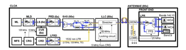
Figure B.3: LO block diagram, showing the Central LO (CLO) and the LO section in the WCA in each front end. Yellow lines represent common synchronization and reference signals fed to all antennas, blue lines are LO signals which are individual to each antenna. For a description of acronyms, see text.
