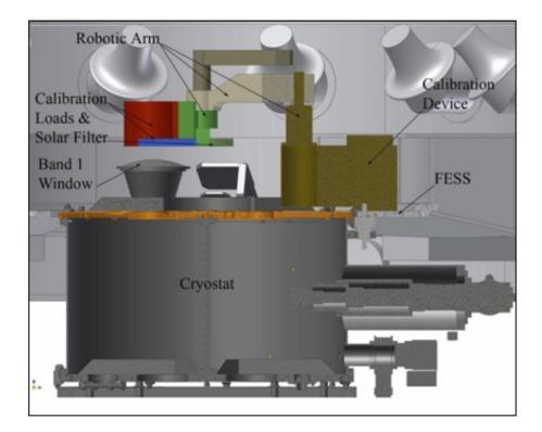
Figure A.7: Lateral view of the ACD on top of the ALMA front ends.
