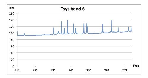
Figure 4.19: Typical  $T_{\rm sys}$  at zenith for Band 6 with 1.262 mm PWV, based on measured values of the receiver temperatures.  $T_{\rm sys}$  was computed using only the receiver temperature values adopted in the OT and the atmospheric contribution. No spill-over or background terms have been included. Temperature is given in Kelvin.
