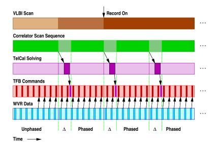
Figure 8.7: VLBI Scans in the Phasing System. Each VLBI scan is partitioned into "subscans" for correlation and "slow" timescale processing (seconds) in TelCal. WVR adjustments are made in the CDP on a "fast" timescale (every second). See text for full discussion and explanation.
