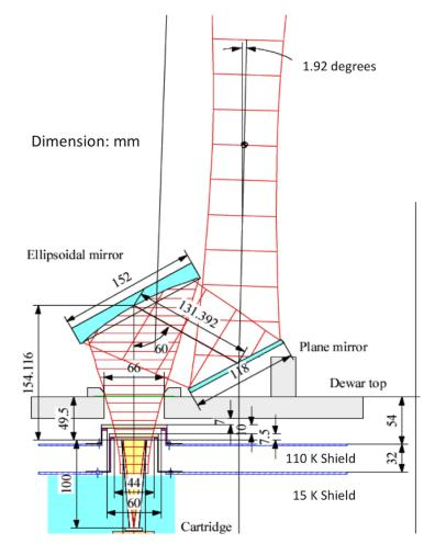
Figure 4.8: Optical layout of the Band 4. Red indicates Band 4 Gaussian beam of 5 times the beam width.
