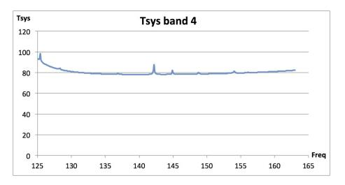
Figure 4.11: System temperature  $(T_{\text{sys}})$  at zenith for Band 4 with 1.262 mm of PWV.  $T_{\text{sys}}$  was computed using only the receiver temperature values adopted in the OT and the atmospheric contribution. No spill-over or background terms have been included. Temperature is given in Kelvin.
