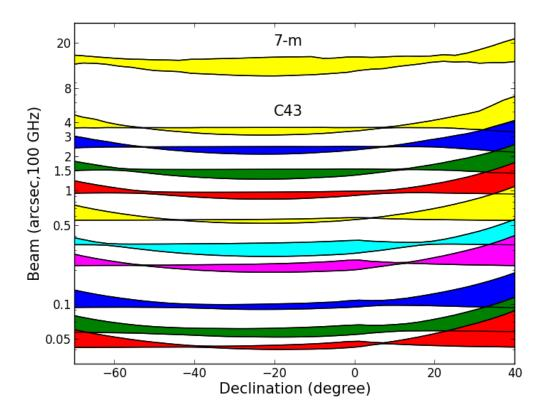
Figure 7.9: Cycle 5 angular resolutions as a function of source declination. Each color shows, for a particular configuration, the range of the major and minor axes of the synthesized beams expected from a 2-hour observation at 100 GHz and at transit. 12-m Array configurations are arranged with C43-1 at the top and C43-10 at the bottom.
