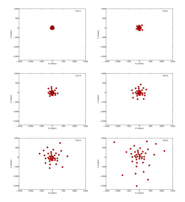
Figure 7.2: Representative 12-m Array compact configurations for Cycle 5.
