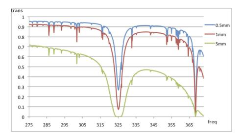
Figure 4.22: Band 7 atmospheric zenith transmission for PWV=0.5, 1.0 and 5.0 mm. Frequency is in GHz. The deep atmospheric absorption at 325 GHz is due to water, and the narrower feature at 369 GHz is due to oxygen.
