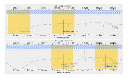
Figure 9.2: A Band 9 spectral setup as displayed in the spectral visual editor in the OT. The top figure shows an example of how the image equivalent of a single spectral window can fall into an area of poor atmospheric transmission, leading to much higher  $T_{sys}$  than necessary. Placing a dummy spectral window at a higher frequency can remedy the situation (bottom).
