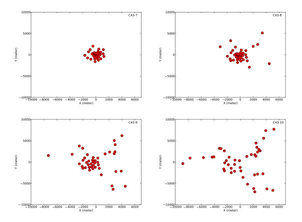
Figure 7.3: Representative 12-m Array extended configurations for Cycle 5.
