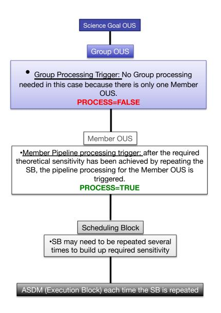
Figure 13.1: Pipeline processing of a Science Goal for single epoch, single array data. The same SB may need repeating N times to build up the requested sensitivity. This Science Goal would result in 1 Pipeline processing, with 1 set of science products delivered to PI.
