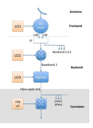
Figure 6.1: Summary block diagram of ALMA signal path and LO system for one spectral window, one baseband, one polarisation. The Backend IF system is located in each antenna, and the digitised signal for each baseband/polarisation is fed to the correlator in the central technical building through buried optical fibers. See Appendix B for a more detailed description of the components and the other tasks that the LO systems perform.
