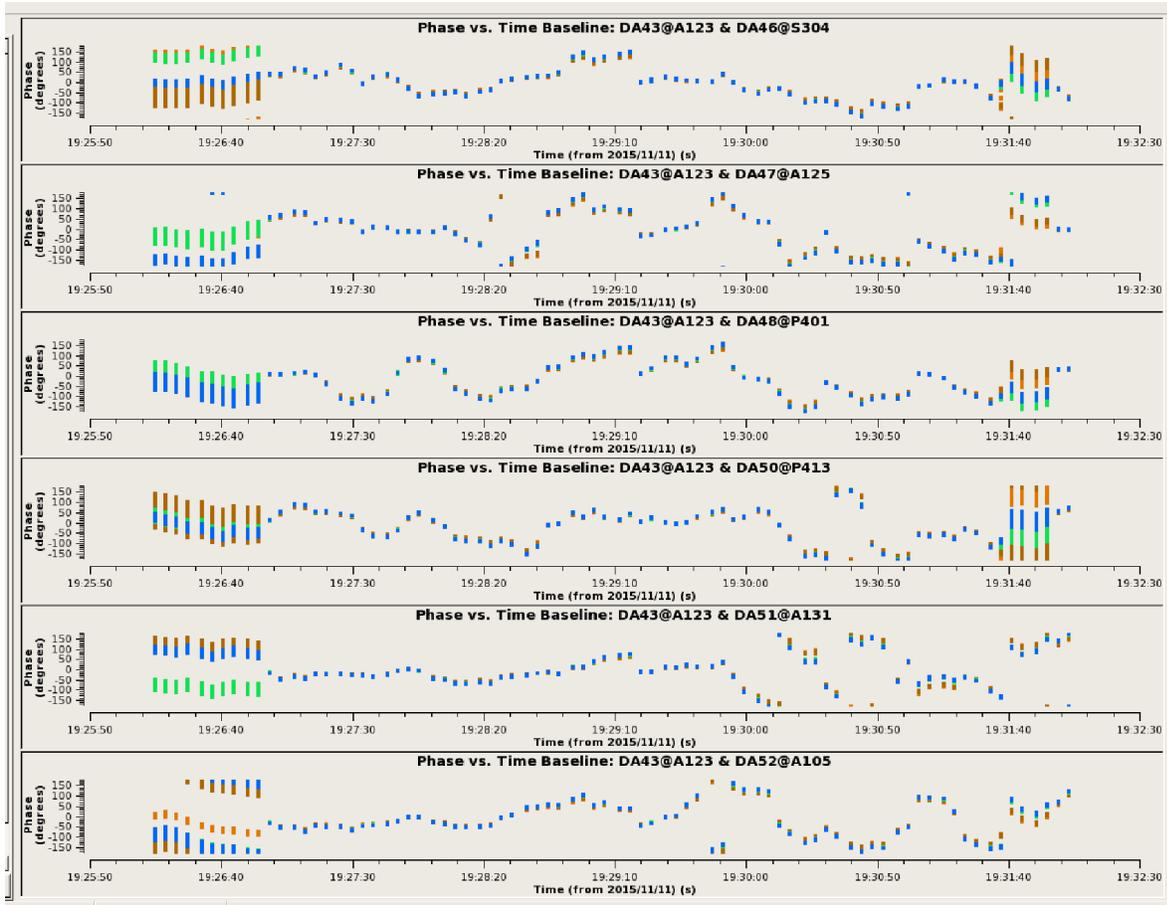
Figure 2: As in Figure 1, but showing several baselines plotted individually. Here, only XX data are shown, and the the four colors correspond to the four correlator quadrants. Once phase-up is achieved near 19:26:55 UT, the dispersion in the phases within in baseband decreases markedly, with values converging near zero phase, as expected. However, the phases subsequently drift, with the four quadrants varying in lock-step. A complete loss of coherence occurs near the end of the scan.
