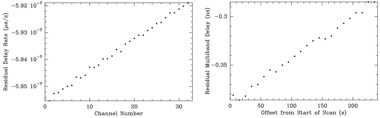
Figure 13: Additional results from the Band 6 VLBI data of April 8, 2017. *Left:* The residual delay rate as a function of frequency channel for the first scan on 3C279 on the ALMA-LMT baseline, LL polarization. There is a linear drift in the residual delay rate with frequency. *Right:* The residual multiband delay found by fringe-fitting different 10-second segments of the data. There is a linear drift of residual multiband delay with time.
