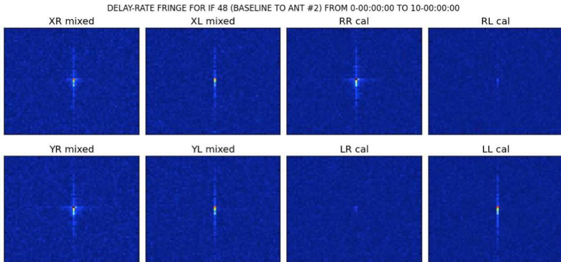
Figure 8: Delay rate fringe amplitudes for the source 3C279 on a baseline between ALMA and the LMT (Band 6). The data were obtained on April 8, 2016. The four left panels show the “mixed” linear and circular polarization products prior to the application of PolConvert. The four right panels show the data after PolConvert. The signal in the cross-hand products is negligible after the conversion, indicating robust operation of the conversion software. From Martí-Vidal et al. (2016a).
