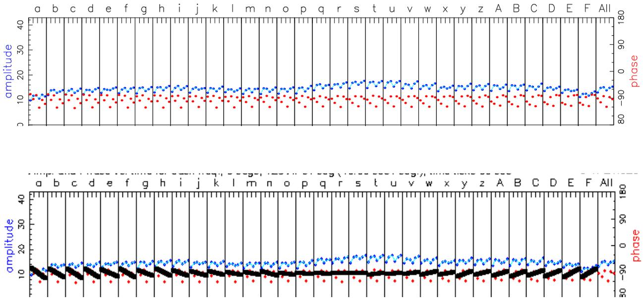
Figure 14: Additional results from the Band 6 VLBI data of April 8, 2017. *Top:* The red points show the phase vs. time on the ALMA-LMT baseline (LL polarization) on the first scan of the experiment for each of the 32 frequency channels (labeled by letter). *Bottom:* The same plot, but with a line drawn in connecting the first and last time points within each channel. The effect of different residual delay rates (i.e., time-varying phases) is evident in each channel.
