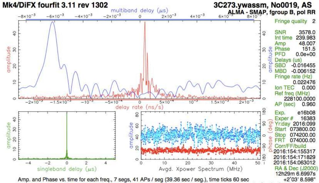
Figure 7: Band 6 (228.1 GHz) VLBI fringe on the quasar 3C273 obtained between phased ALMA and the phased SMA on April 8, 2016. The plot shows a correlation between ALMA’s X polarization and the SMA’s R polarization based on 4 minutes of data.
