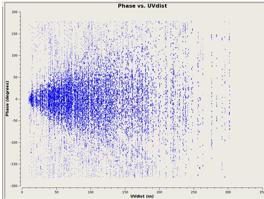
Figure 11: Phase as a function of  $u-v$  distance for the same Band 6 data as shown in Figure 10. Scatter in the phases increases systematically with increasing baseline length. Data source: uid://A002/Xb187bd/X2d5.
