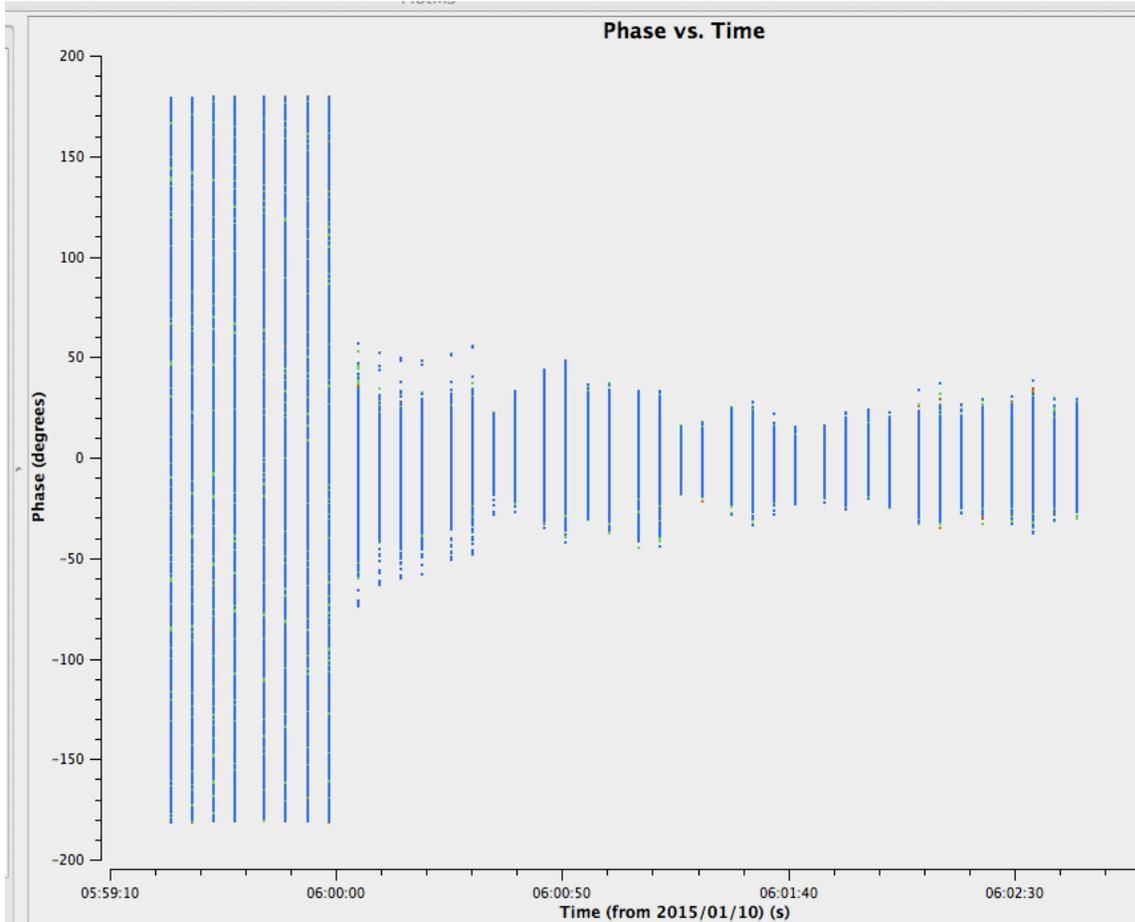
Figure 3: Phases as a function of time during a 3.5-minute Band 3 observation of the quasar 0730-116 with the ALMA phasing system on 2015 January 9. The baselines for 41 antennas that received phasing corrections are plotted (polarization XX). Each of the four correlator quadrants is shown in a different color (although the symbols overlap). Phase-up (i.e., the expected convergence of the phases toward zero for an unresolved source) is clearly observed in all four quadrants.
