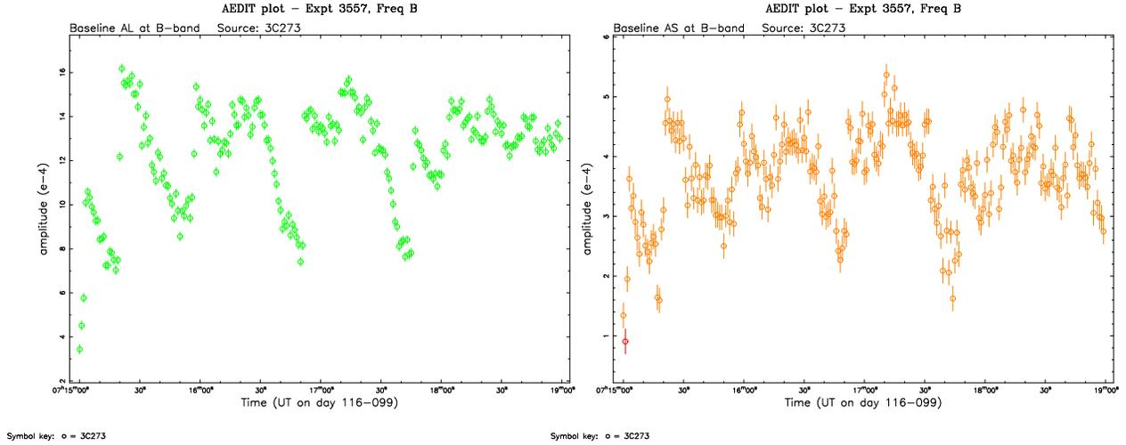
Figure 9: Amplitude vs. time during a Band 6 VLBI scan on 3C273 for the ALMA-LMT (left) and ALMA-SMA (right) baselines, RR polarization, obtained on April 8, 2016. The correlation coefficients are seen to decay frequently, reflecting a loss of phasing efficiency, but then recover to a nominal level. These dropouts occur at the same time on two different ALMA baselines, indicating that the issue originates at ALMA.
