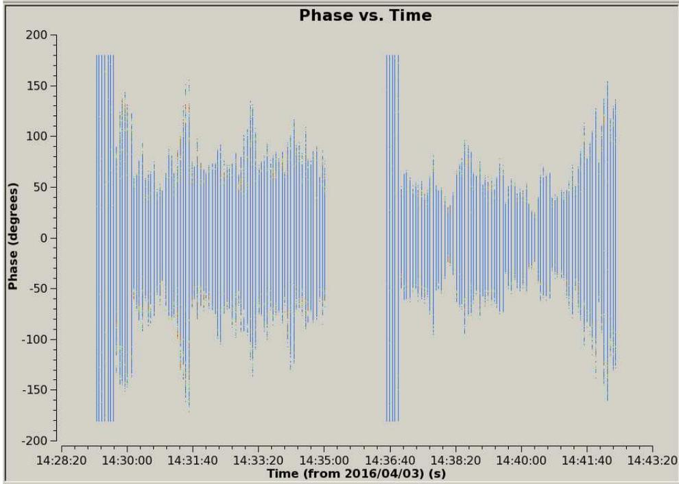
Figure 5: Band 3 regression test data obtained with the APS on April 3, 2016 using the Cycle 3 software release. Phase is plotted as function of time for all four correlator quadrants, XX polarization. While the scatter in the phases is high, it appears to be consistent with the unstable weather conditions. There is therefore no evidence for the types of phasing problems seen in test data from November 2015 and March 2016 (cf. Figures 1-4). Data source: uid://A002/Xb1586e/X4b2f.
