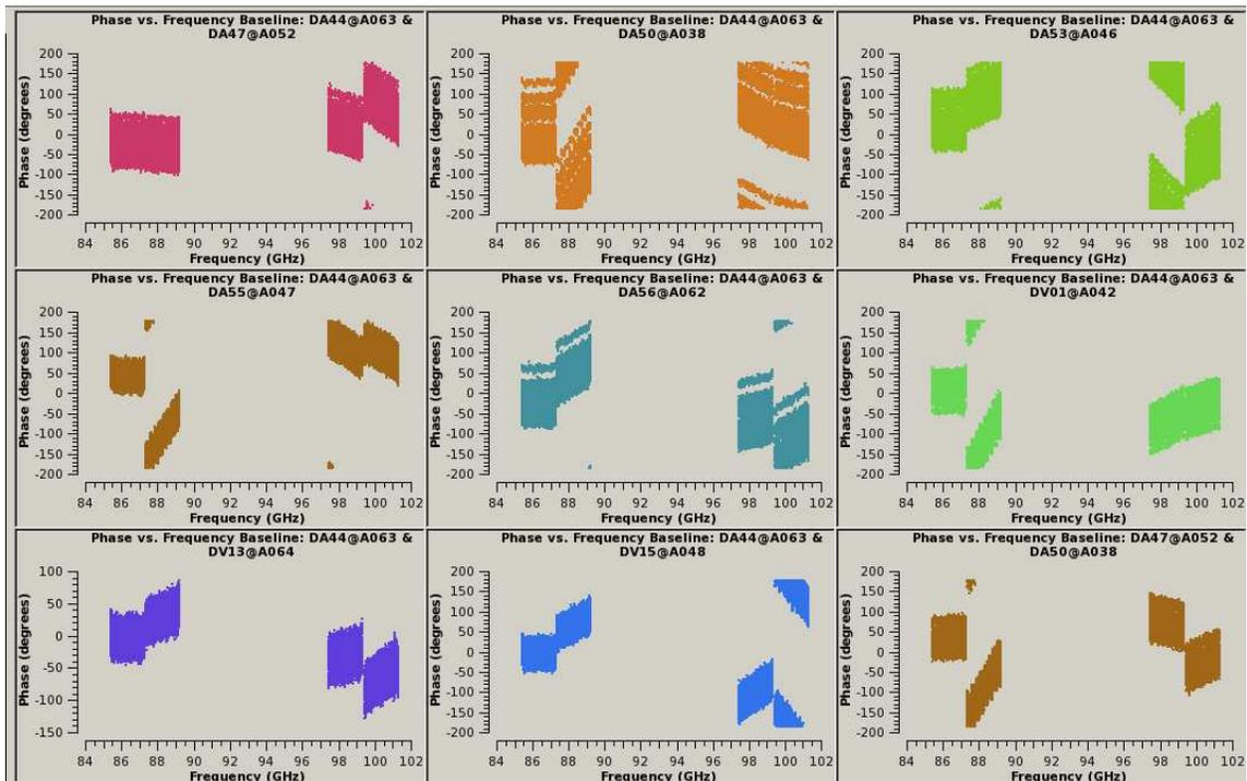
Figure 6: Band 3 test data obtained with the APS on April 3, 2016 using software release R2016.6. In each subpanel, phase is plotted as function of frequency for all four correlator quadrants, XX polarization, during a single scan on a baseline between phased antennas. Phased slopes are visible in several of the panels, indicating delay errors. Data source: [uid://A002/Xb16072/X1cc](http://uid://A002/Xb16072/X1cc).
