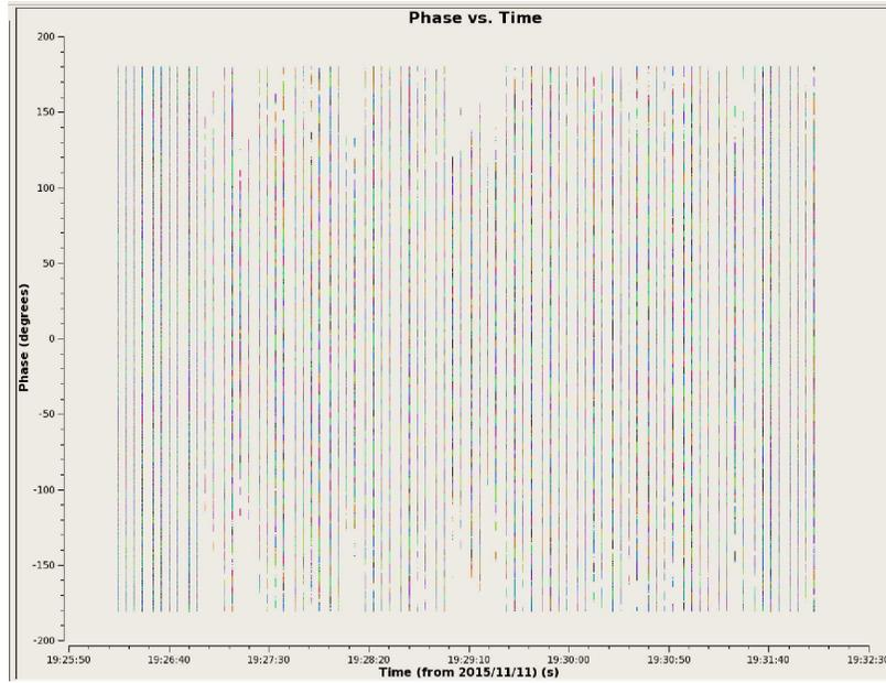
Figure 1: Band 3 observations with the APS obtained on November 11, 2015. The target was the bright quasar 1924-292. Phase as a function of time is plotted for data for baselines between all phased antennas (37 in total) from the first correlator quadrant, XX and YY polarizations. Approximately 360 seconds of data are shown. Data source: [uid://A002/Xacba6b/X15](http://uid://A002/Xacba6b/X15).
