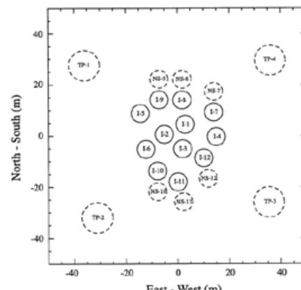
Fig.3. The locations of the ACA 7m Interferometer (I) and ACA 12m Total Power (TP) antennas. The four TP antennas will remain at fixed locations under normal operations. The smaller dashed circles mark the locations of the ACA 7m antennas when these are used to measure sources at northern declinations. This more spread-out arrangement reduces any blockage of the inner antennas by outer antennas.
