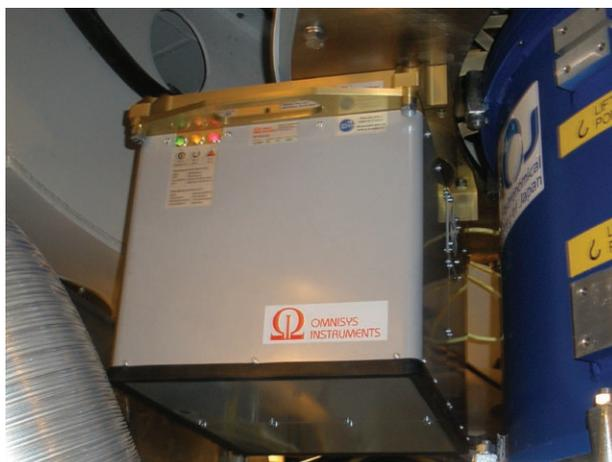
*Figure 4. A water vapour radiometer installed in the receiver cabin.*
