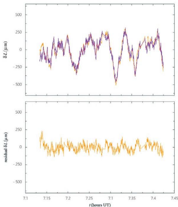
Figure 10. Phase Correction on a mm source. In the upper plot the red line is the raw phase of the astronomical signals (converted into a path difference), and the blue line is the difference as measured by the radiometer, while the lower plot is the residual after applying the correction. (Credit Bojan Nikolic)
