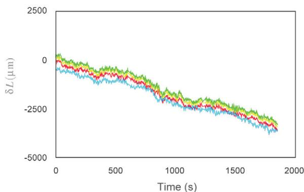
Figure 8. Additional path due to water vapour from three different antennas. (Credit Bojan Nikolic.)
