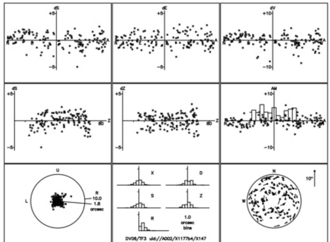
Here is the analysis (made with the TPOINT™ package from Patrick Wallace) of such an interferometric pointing run demonstrating conformance with the ALMA requirement of 2 arc second rms accuracy over the whole sky.
