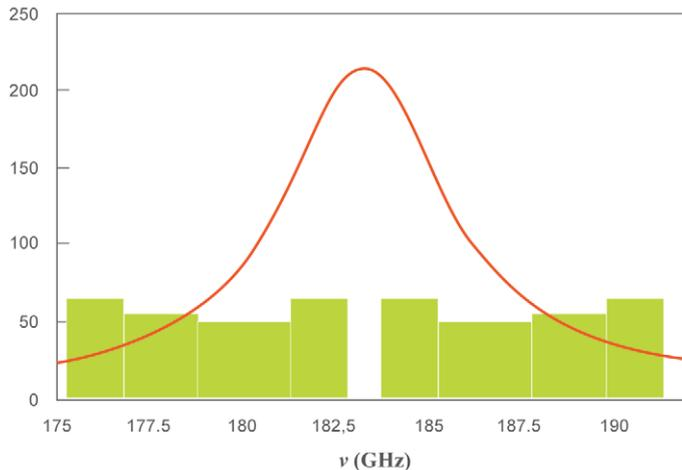
Figure 7. Close up of the 183 GHz emission line of water vapour and the frequency coverage of the channels of the radiometer. (Credit Bojan Nikolic.)
