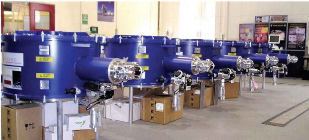
*Fig.2 A photo of the cryostat that houses the SIS mixers and amplifiers. The SIS mixers must be cooled to 4 degrees above absolute zero to function optimally. The amplifiers following the SIS mixers are not cooled to such a low temperature, but these are also extremely low noise systems.*
