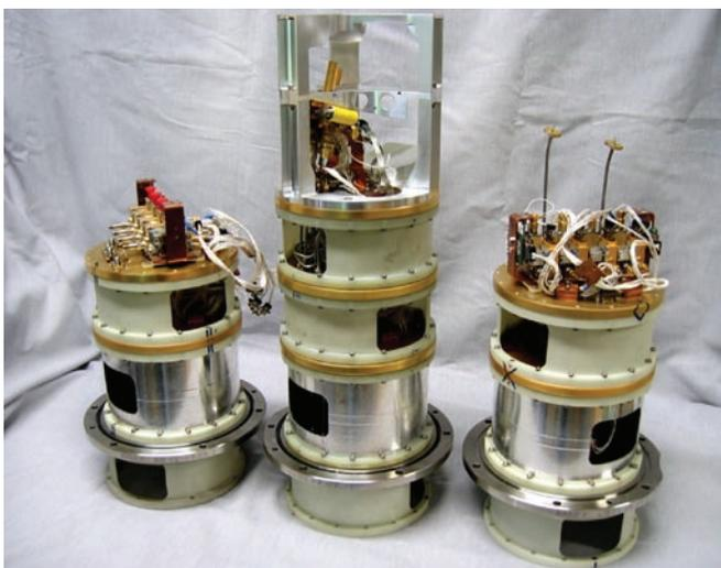
*Fig.1 A photo of three Band 7 prototype front ends in various stages of construction. These are superconducting mixers (SIS) that efficiently convert the power at the sky frequency to a much lower intermediate frequency (IF) where the power is amplified greatly. The advantage of the SIS mixers is that these have contribute an extremely low noise, give rise to only very small losses in the input power and require only a small amount of local oscillator power.*
