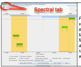
Figure 11: A graphical view of the correlator setup using the Spectral tab, showing the ranges for each baseband as well as the bandwidth and range of each spectral window.
