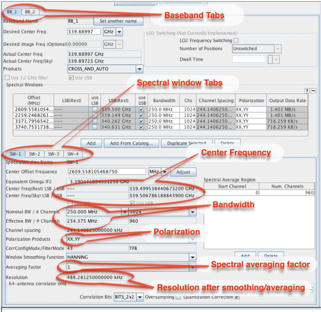
Figure 10: Click on the Science Instrument Setup and scroll to the bottom of the Editor window in order to check your correlator setup. Each baseband (BB) has its own tab, and each spectral window (SW), if more than one within the baseband, has its own tab. Click on each in turn to check the setup for each spectral window in each baseband.
