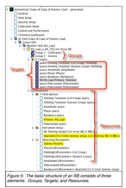
second (or subsequent) Group contains the science targets plus relevant calibrators (e.g. phase, atmosphere, pointing, etc.) which are repeated until the science integration time is completed. If you click on a group, then the targets associated with that group are highlighted in yellow.
