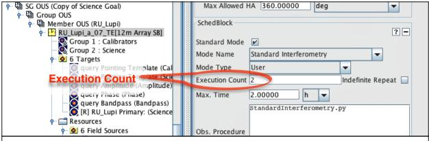
Figure 13: Click on the SB name (yellow clock icon) and scroll down the Editor window to find the Execution Count. The total time on source will be the Integration Time on Source (Figure 12) multiplied by the Execution Count.
